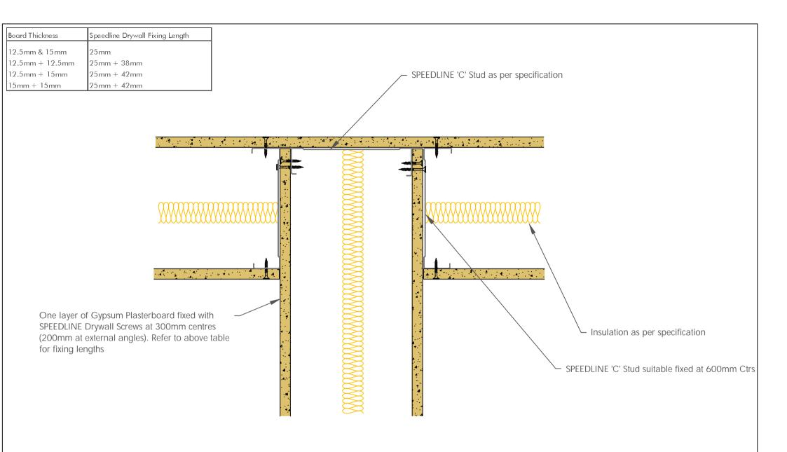
DATE: 21/02/19 CDR No: 317 SCALE: NTS C STUD ACOUSTIC T JUNCTION DETAIL
