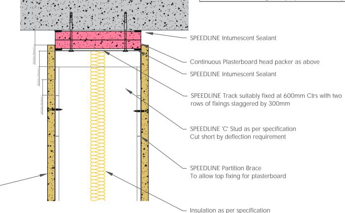
One layer of Gypsum Plasterboard fixed with SPEEDLINE Drywall Screws at 300mm centres (200mm at external angles). Refer to above table for fixing lengths
